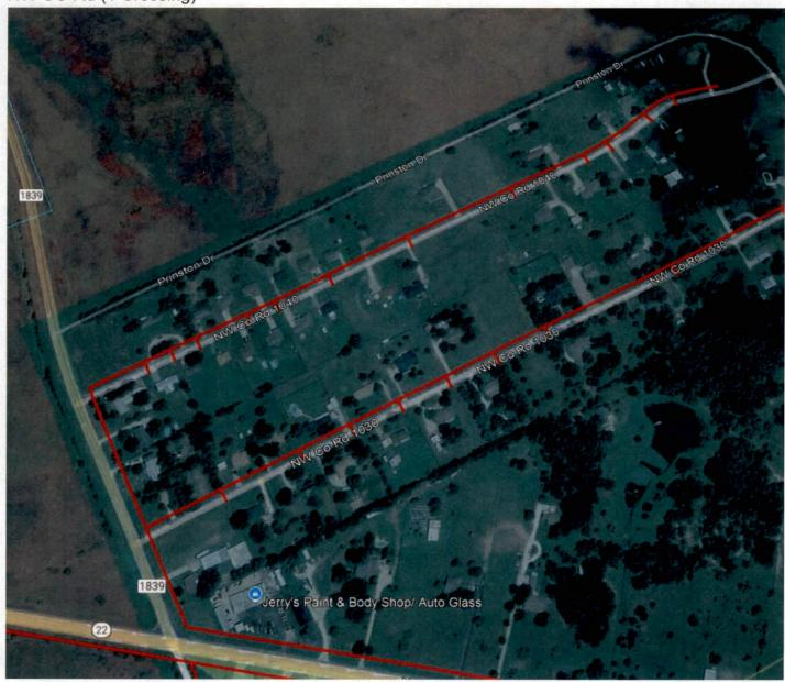
County Roads B27 Pt 2(Green Shade) Precinct 1 Red lines indicate underground directional bore path White lines indicate Aerial placement on existing poles. Drane Rd
